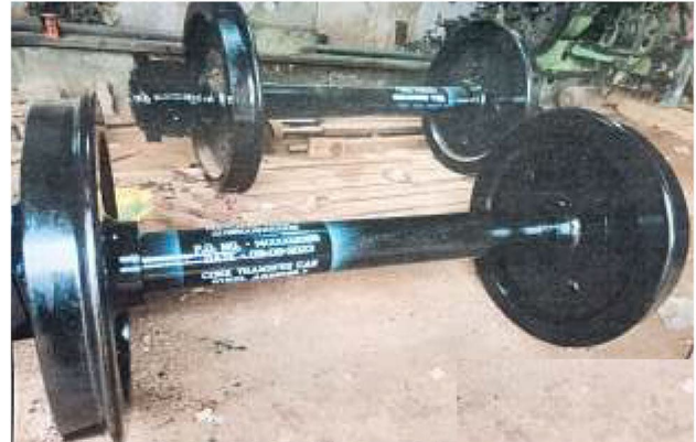
Coke Transfer Wheel Assembly
