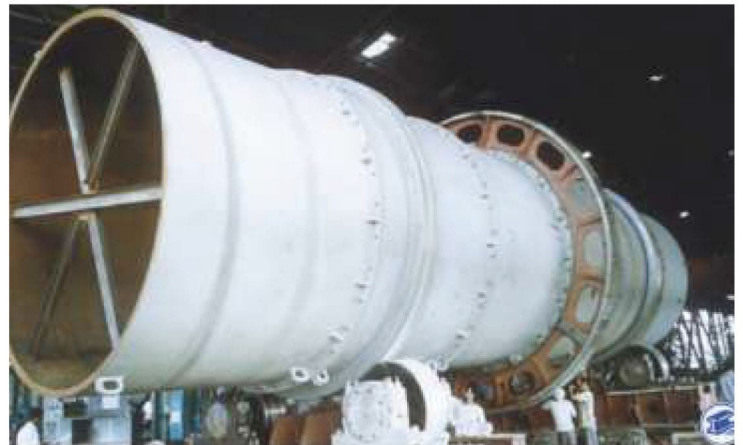
Balling & Mixing Drum of Sinter Plants
